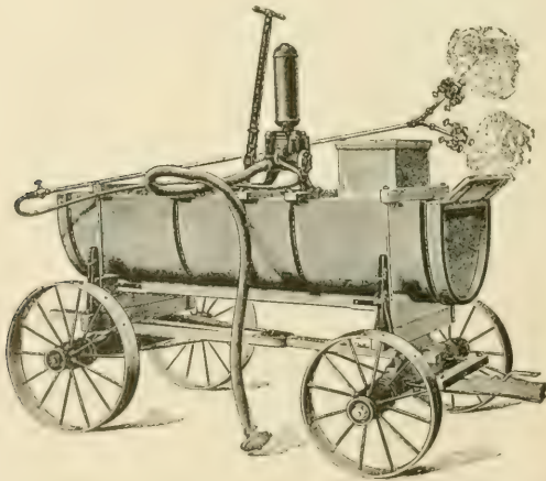
FIG. 36—Double-acting horizontal pump mounted on 250-gallon tank. A good type of outfit for medium sized commercial orchards. (Va. Agr. Exp. Sta.)
